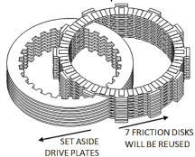
Inspect the friction disks for signs of heat or wear. Replace if they are burnt or worn. For most models, new friction disks can be purchased from Rekluse.
