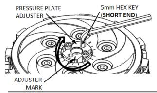
**NOTE:** As you turn the adjuster, the clutch may slip and start to spin before you reach 1-full turn. With the bike in gear you can hold the rear brake for leverage.
