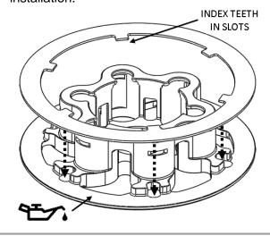
12. Install this pressure plate subassembly.
