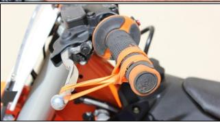
With the bike at idle in neutral, quickly blip (rev) the engine to at least 5,000 RPM and let it return to idle. The clutch lever should move in about 1/8" (3mm) toward the handlebar as you rev the engine.
