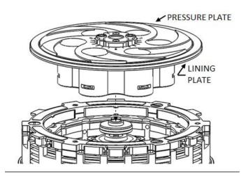
13. Install the pressure plate springs.
