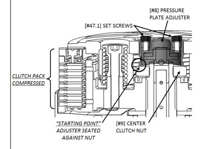
17. Now, insert the **short end** of the 5-mm hex key into the pressure plate adjuster, and turn it clockwise **one full turn plus 2 tick marks past the starting point** (aka "1+2").
