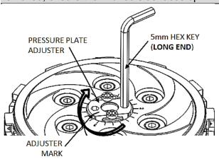
**15.** At this point, make a note of where the mark on the adjuster aligns with the tick marks on the pressure plate. This is your **starting point.**
