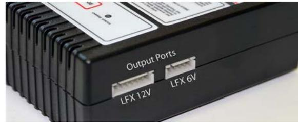
At this point you should have the battery charge cable connected to the battery BMS port, and the AC input cord connected to the charger. Now insert the AC plug into an appropriate AC wall socket. Whenever possible, use the charger's retractable hook to hang the BMS01 above the floor, in a location which allows easy access to the battery charge cable. Now plug the battery charge cable into the correct LFX charge output port (or into the extension cable).
