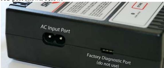
Note that the small 3-pin port to right of the AC Input is reserved for factory diagnostics, and should never be used, modified, or have anything attached to it.
