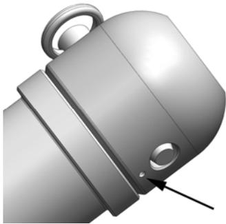
3) Install the plastic top using the removable pin. **Important:** One side of the puck has a small hole drilled beneath the main hole. Install the pin so that the end of the pin with the ball is on the same side as this small hole. The pin should be installed so that the ring is on the top half of the slider.
