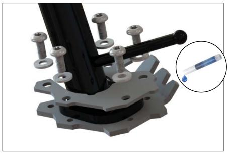
Take the (5) screws and add the washers and a small drop of thread locker to each screw.
