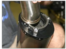
Install TBR muffler assembly to motorcycle with the rubber lined muffler clamp on muffler and barrel clamp on slip-tube.
