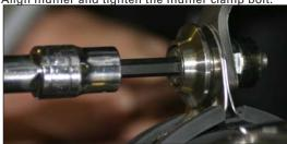
8. Check alignment and tighten X-Ring bolts then barrel clamp.
