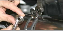
7. Align muffler and tighten the muffler clamp bolt.
