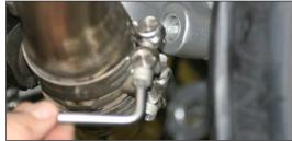
Install supplied muffler mounting bracket using the 8x20mm bolt that is provided.
