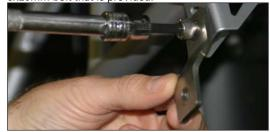
Loosely attach TBR slip-tube to TBR muffler using the supplied two-part X-Ring and 6x20mm bolts with lock washers, use supplied lock-tight.
