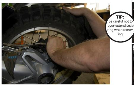
Place the bike on its side stand. Using your hand compress the rear brake caliper so you can freely move the rear brake lever down.
