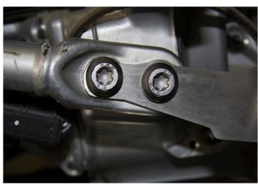
NOTE: If you also purchased AltRider crash bars install them first, reference crash bar instructions and take note that step #1 is critical. If you already have AltRider crash bars installed skip to step #3. Place bike on center stand. Remove OEM skid plate and any brackets. Using a T50 Torx driver remove the (2) OEM engine bolts from each side, keep them.
