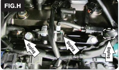
13 Unplug the stock wiring harness from all three of the bike's Fuel Injectors (Fig. H).
