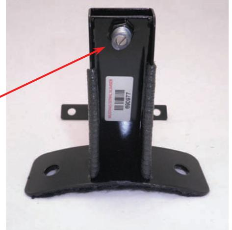
The tilt angle, forward and back, is controlled by a chromed thumbscrew at the front of the driver backrest post. Turn clockwise to tilt forward, counter-clockwise to tilt back.
