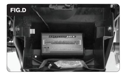
Using the supplied Velcro, secure the PCV module in the rear section of the trunk (Fig. D).
