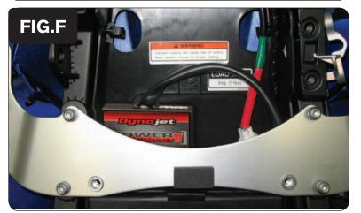
8 Install the PCV in the tail section of the bike using the supplied velcro (Fig. F). It is recommended to route the PCV harness underneath the subframe bracket. Make sure to use the alcohol swab to clean both surfaces before attaching velcro.
