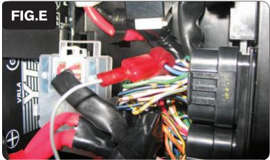
7 Using the supplied posi-tap attach the GREY wire of the PCV to the BLUE wire of the ECU (Fig. E).
