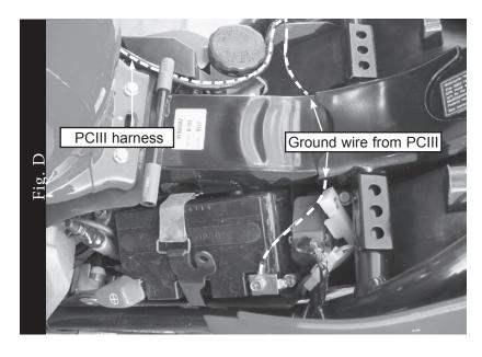
Route the ground wire from the PCIII harness under the frame towards the battery. Attach ground wire from PCIII to the NEGATIVE terminal of the battery (Fig. D).
