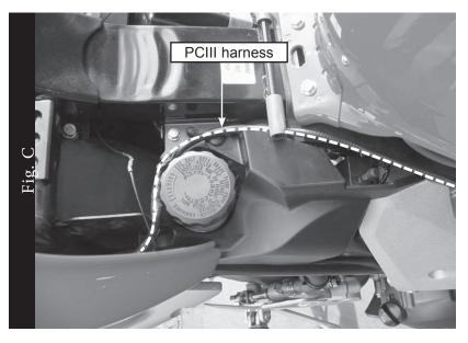
Route the PCIII wiring along the inside of the frame towards the rear of the bike (Fig. C).
