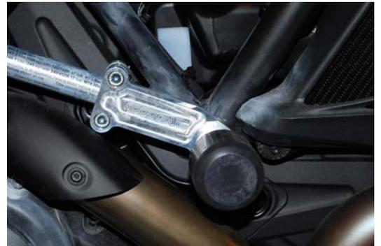
10) Slide the plastic slider over the top of the base and secure in place using the 8 mm countersunk bolt provided. The bolt passes first through the non threaded hole and then screws into the threaded hole on the far side of the base. The plastic is undersized on the far side of the slider to act as a locknut for the bolt
