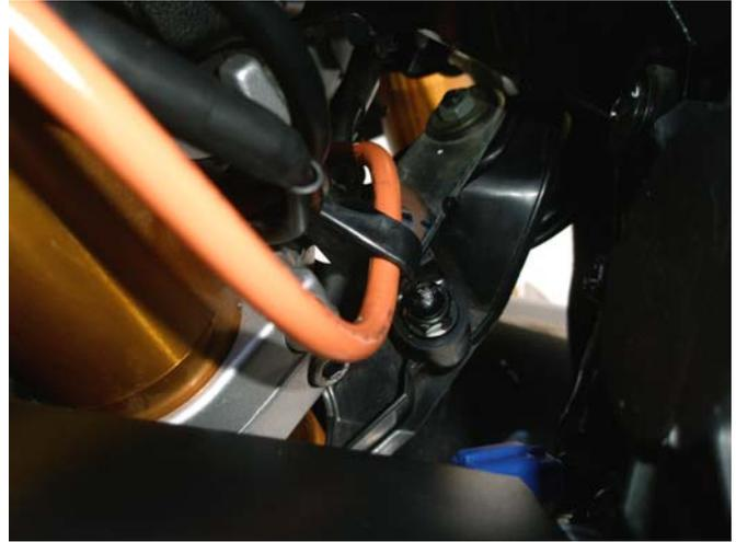
**b. Routing from master cylinder, top of the lower triple tree**
