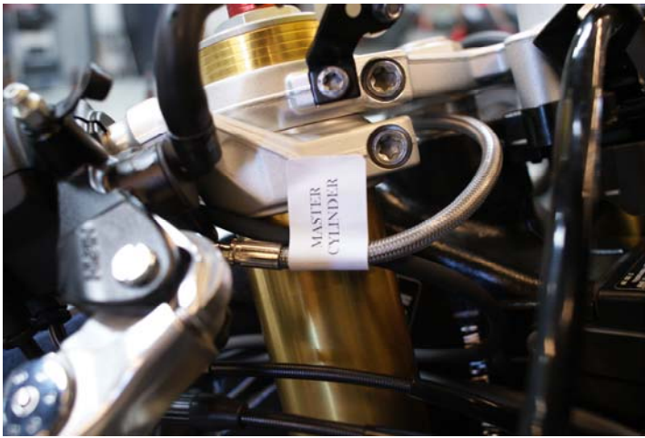
a. Line A, front master cylinder
