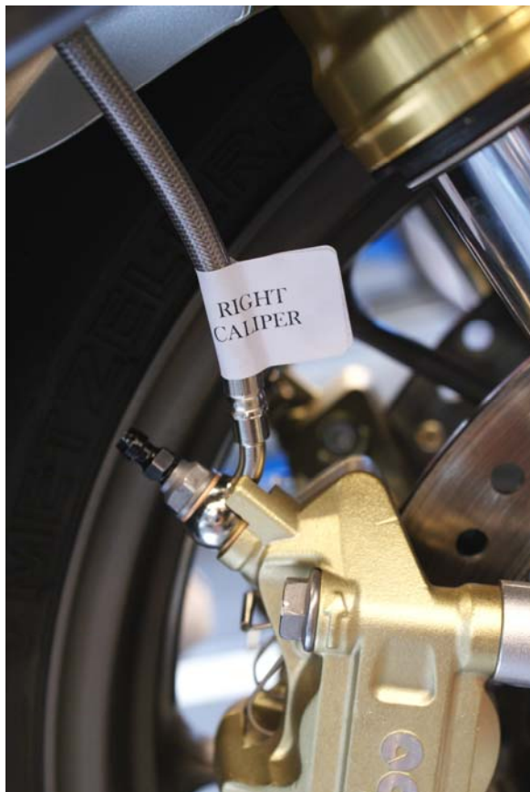
i. Line B assembly, Right Line at right caliper with OEM bleeder bolt
