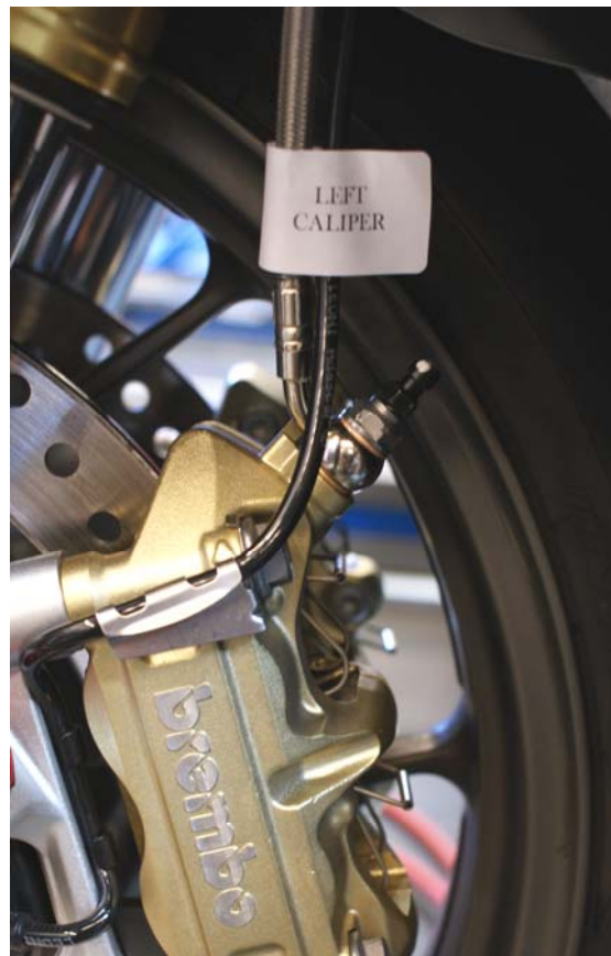
j. Line B assembly, Left Line at left caliper with OEM bleeder bolt
