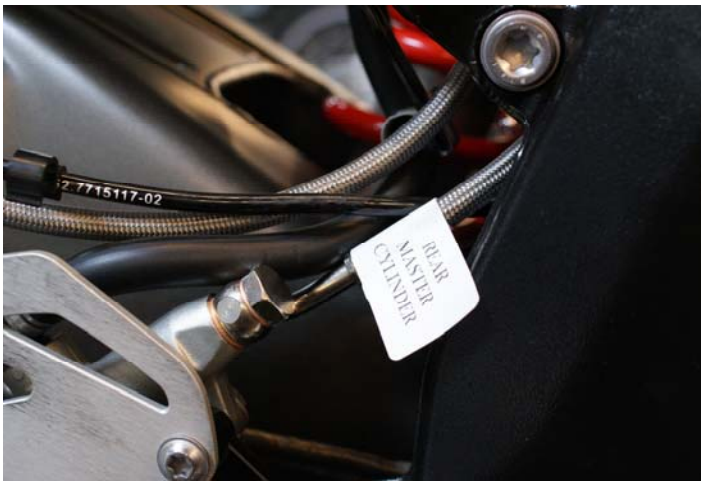
m. Line C, rear master cylinder
