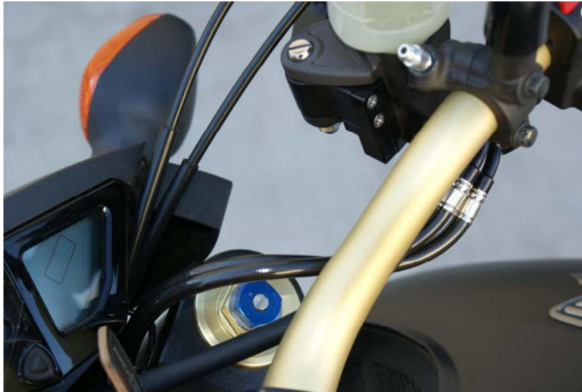
E. Lines routing from Master Cylinder down through stock guide bracket
