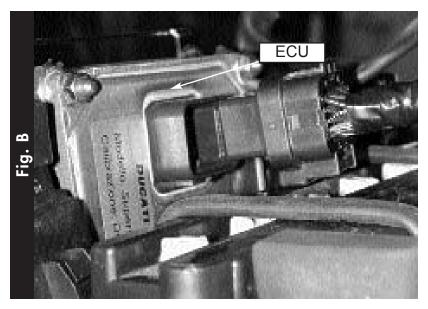
4 Plug male connector from PCIII into ECU (Fig. B).
