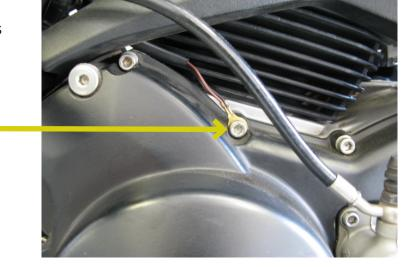
13. The Monster is equipped with two lambda/O2 sensors. These sensors must be bypassed through the use of O2 eliminators supplied with the kit. Disconnect the factory harness connector from each sensor. Install the Bazzaz O2 eliminators in place of the factory sensor connectors and attach the O2 eliminator ground lugs to chassis ground. Be sure to secure the eliminator and factory sensor lead away from any hot or moving components which could cause damage to the components.
