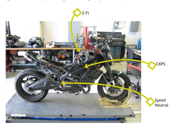
2. Mount the control unit on top of the factory ECU using a supplied cable tie. Connect the Bazzaz fuel harness main connector to the control unit and begin to route the harness down the right side of the engine.
