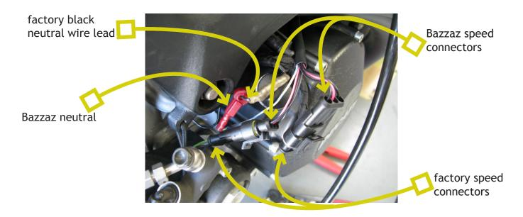
8. Route the Bazzaz power connector (Orange Label) along with the factory harness towards the rear of the motorcycle. Locate the **yellow** wire coming out of the small eight pin connector on the right side of the tool tray. Crimp one of the supplied scotch lok connectors onto this **yellow** wire and insert the Bazzaz power connector (red connector with red wire) into the scotchlok.
