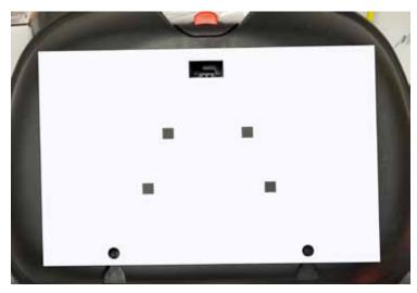
Using the cleaning pad provided, clean the surface of your Givi box. Align the template (from the next page) to place the provided bumpers. This ensures they land in the right spots on the rack.
