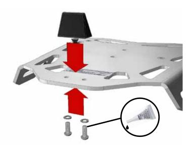
Assemble the lock tower as shown. Apply one drop of thread locker (included) to the last couple of threads of the two fasteners before inserting them.
