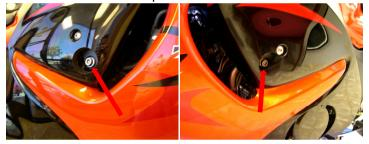
9. Remove right side bolt. Mount right side puck with (99-HB-SH10125090) Socket Cap 10 X 1.25 X 90 Main Engine Stud and torque down.
