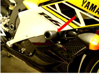
4. Remount right side body panel, line up the notch with the panel to clear.
