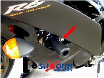
6. Mount Left side slider to the offset using 99-HB-SH10150045 Socket Cap 10 X 1.5 X 45 (Holds puck to offset). Use one drop of blue thread locker and torque down to 30 to 32 foot lbs.
