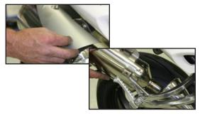
Loosen stock O<sup>2</sup> sensor and barrel clamp and remove the rear s-bend section.
