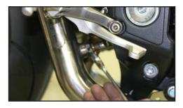
Make sure position of muffler is correct. Once you are satisfied with its position, tighten X-Lite™ ring bolts on the V.A.L.E.™ assembly.
