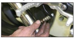
9. Position s-bend so that it clears on all sides and then tighten bottom clamp.
