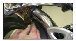
Tighten the muffler clamp, securely attaching the muffler assembly to the bike.
