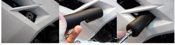
17. Mount right side puck using 10 X 1.5 X 90 (99-HB-SH10150090) bolt and washer. There is a cutout in the puck to clear the body orientate the puck and torque down to 35ft lbs.
