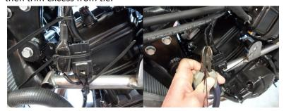
14. Loosely mount the counter shaft sprocket cover to create a clearance pattern. Once you have created clearance for the left side rail mount the counter shaft cover and tighten up.
