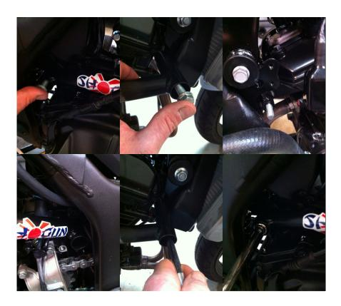
12. After mounting the rails in step 11 install each of the 4 round finishing plugs (99-CP-4120) into each open end of the Shogun rails.
