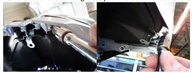
7. Remove left and right upper cowls and unclip turn signal plugs.
