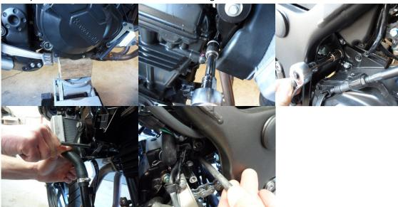
10. Remove left side harness bracket. Note: The rubber coated connector has to be unplugged to be removed from bracket the other unclips from the bracket.
