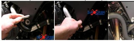
6. Remove the bodywork and double check location of spot mark the tool has created.
