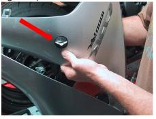
11. Remove right side bolt. Mount right side puck with (99-HB-SH12125090) Socket Cap 12 X 1.25 X 90 Main Engine Stud and torque down.
