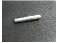
With the body removed, thread in by hand your spot tool. Make sure you have the spot tool screwed in enough to clear the body on the inside.
