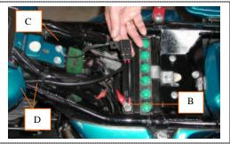
**STEP #3** – Finish routing the wire under the tank and up to the horn bracket. Install the fuse in the fuse-holder. The center terminal is plus and the outer ring is negative (see dwg below). Apply either dielectric grease or Vaseline to the spade terminals. Connect the red wire to the positive spade terminal & the black wire to the negative terminal. Use a voltmeter to check if the polarity is correct.
