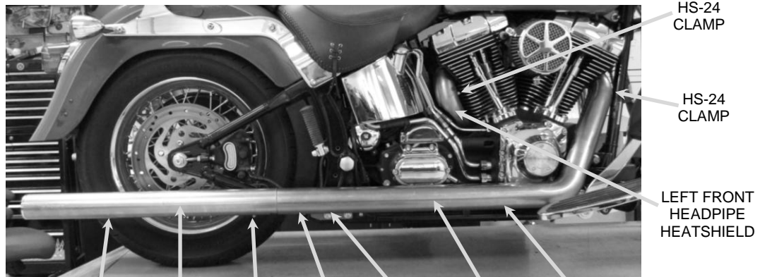
NOTE: Arrows point to the position of the hex head of the clamps. HS-28 CLAMP RIGHT MUFFLER HEATSHIELD HS-28 CLAMP 27-61MSC CLAMP HS-24 CLAMP RIGHT FRONT HEADPIPE HEATSHIELD HS-24 CLAMP FIGURE 6
