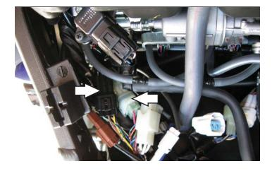
7 Unplug the two different 6-pin connectors from the throttle bodies.
