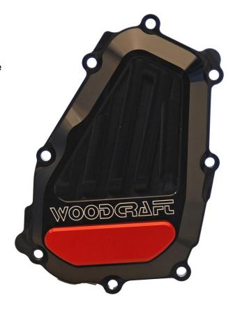
3) Attach the pickup and wire retainer using the OEM hardware to the Woodcraft cover.
