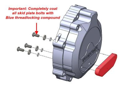
The generic cover at the right shows both o-rings and optional washers on the skid plate bolts. If your skid plate did not come with washers, simply put the o-ring directly beneath the head of the bolt.
