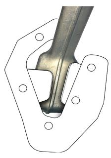
With bike on the center stand, arrange the top and bottom plates identically to how they are shown in the picture to get an idea of the fitment. Leave top plate resting on side stand.
