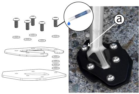
Take the (5) screws and add the washers and a small drop of thread locker to the end of each screw. Note which fastener gets the stack of washers (placed between the two plates), indicated as (a) above. Now match up the bottom plate to the top plate and install all (5) screws with washers.
