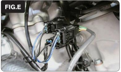
10 Plug the PCV wiring harness in-line of the stock Gear Position Sensor connectors (Fig. E).
