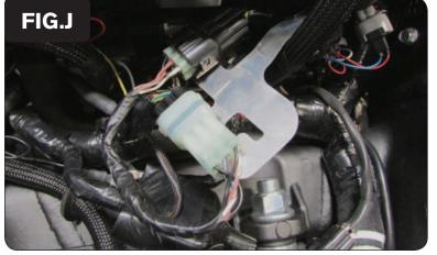
Plug the PCV wiring harness in-line of the each Fuel Injector and each of the stock wiring harness connectors (Fig. G).
