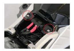
If the front of the seat is not tight in the front mount or if the rear bolt will not line up, the motorcycle's front mounting bracket can be adjusted by loosening the two Torx screws with a T-30 bit and repositioning the bracket. Re-tighten the Torx screws securely before mounting.
