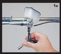
Tools and supplies needed: 1) 4mm allen wrench, 1) 10mm wrench or socket 1) small cleaning rag.
