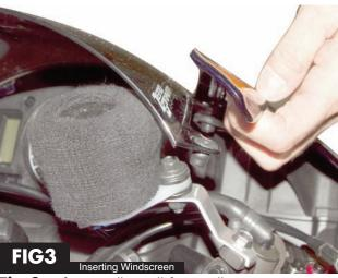
**Fig 3.** After installing all four well nuts on your new ZG windscreen, insert the windscreen from the backside and slide the windscreen forward, lifting the upper fairing as shown.
