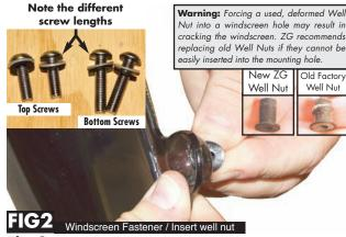
**Fig 2.** Note: The screw bolts are different lengths. To reuse factory well nuts, lubricate the four well nuts with soap or saliva and insert them into ZG screen from the backside as shown above. **Note:** If old factory well nuts are deformed (as shown above) you may want to change them out with our ZG well nut kit part #32-111.
