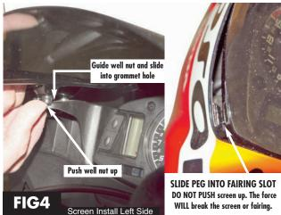
**Fig 4.** While lifting the upper left fairing with one hand slide/push left side of the bottom wellnut first, into grommet hole as shown above. Simultaneously inserting the front windscreen, slide peg into the fairing slot.
