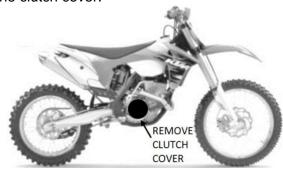
2. Remove the OEM parts named in the following diagram. Note the orientation of the Bellville spring and quantity of clutch plates removed.
