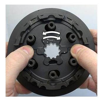
**7.** Remove the 6 rubber dampers from the OEM center hub assembly.
