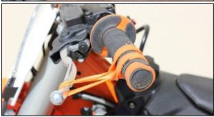
With the bike at idle in neutral, <u>quickly</u> blip (rev) the engine to at least 5,000 RPM and let it return to idle. The clutch lever should move in about 1/8" (3mm) toward the handlebar as you rev the engine. Turn the Slave Cylinder adjuster screw clockwise 1 tick at a time until optimal clutch lever movement (i.e. Free Play Gain) is achieved.
