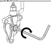
**29.** Once you have found the starting point, turn the adjuster clockwise 1 full turn plus 5 marks (or "1+5"). **This is NOT your final setting**, but it is a good reference point for using free play gain to find the correct setting.
