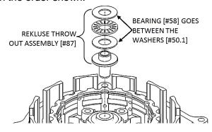
Husqvarna 125cc ('14 and newer) & KTM 125/144/150/200cc ('06 & newer): Install the included throw out spacer onto the
