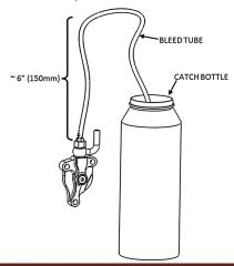
**23.** Pump the clutch lever 3-5 times then hold it against the bar/grip.
