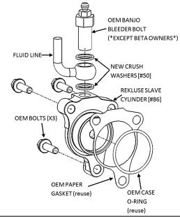
**NOTE:** Some models have a paper gasket and/or O-ring seal. Reuse them if OEM equipped.\***BETA OWNERS:** Use the supplied banjo bleeder bolt in place of the OEM banjo bolt.
