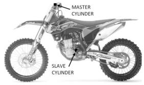
**16.** Starting at the slave cylinder, remove the OEM parts named in the following diagram beginning with the banjo bolt.
