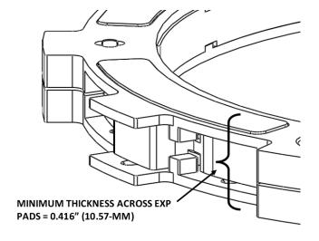
Repeat the break-in procedure anytime the friction disks or EXP bases or wedges are replaced. Always soak friction disks or EXP bases in oil for at least 5 minutes before installing.
