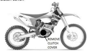
**2.** Remove the OEM clutch parts named in the following diagram. Leave the basket installed.
