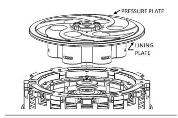
13. Install the pressure plate springs.
