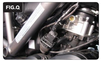
21 Plug the pair of 3-pin connectors of the PCV wiring harness in-line of the stock Crank Position Sensor connectors (Fig. Q).
