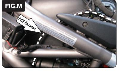
17 Continue routing the PCV wiring harness up the left side of the airbox, then downward, and across to the front-right side of the engine (Fig. M).
