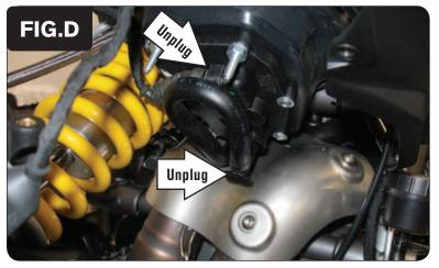
5 Unplug the fuel line and the electrical connector from the bottom of the fuel pump (Fig. D).
