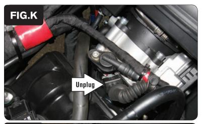
On the rear cylinder throttle body unplug the stock wiring harness from the Fuel Injector (Fig. K).
