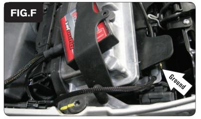
9 Lay the PCV module on top of the ECU temporarily and secure the PCV ground wire with the small ring lug to the negative (-) terminal of the bike's battery (Fig. F).
