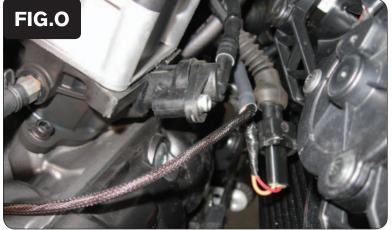
Plug the pair of PCV leads with ORANGE colored wires in-line of the front Fuel Injector and the stock wiring harness (Fig. O).
