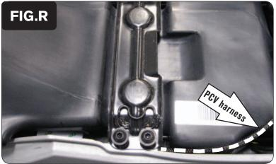
Use the supplied zip-ties to secure the PCV wiring harness where you may see fit.
