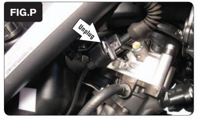
20 Unplug the stock Crank Position Sensor connectors (Fig. P).
