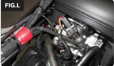
16 Plug the pair of PCV leads with YELLOW colored wires in-line of the rear Fuel Injector and the stock wiring harness (Fig. L).
