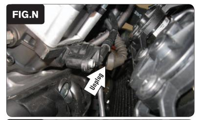
On the front cylinder throttle body, unplug the stock wiring harness from the front Fuel Injector (Fig. N).
