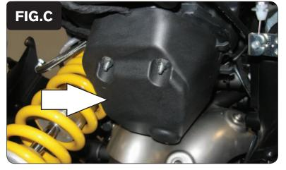
Remove the cover under the tail that covers the fuel pump at the bottom of the fuel tank (Fig. C).
