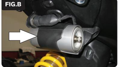
Unbolt and loosen the rear shock reservoir from the under-tail by removing the 2 bolts (Fig. B).
