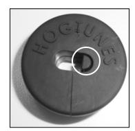
The supplied grommet is "split" to make installation much easier once the wire is in the bag. In the above picture, the white circle is showing a "plug" that can easily be removed. If the only wire you have going into your saddlebag is the speaker wire, leave the plug in place. If you have a second wire for such things as USB power, or a music device interface, removing the plug from the grommet will allow the second wire to also pass without having to drill additional holes in your saddlebag.
