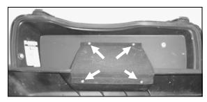
Remove the 4 screws (highlighted with white arrows above) that hold the cloth flap in place. With the flap off ,slide one of the metal bars out from inside the flap as it will be used for new lid. The screws just removed will be re-used.
