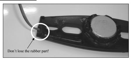
NOTE: Do not paint the tweeter bridge! The tweeter is permanently attached to the tweeter bridge assembly to make sure nothing obstructs the built in drainage. In the event of warranty, Hogtunes replaces the tweeter and the bridge as one piece, and therefore assumes zero responsibility for paint!
