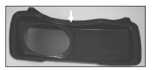
With the gasket installed, you will insert the factory metal strip (5 screws) between the gasket and new lid. Re-install the 5 factory machine screws the same way they came off the factory lid. The new lid will now be attached to your saddlebag.
