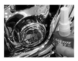
2. Using the supplied hardware and blue Loc-Tite, install the Brouhard points cover using a 9/64 inch allen wrench for Lefty series and a 3/32 inch allen wrench for Waterfall series. Torque to factory specs.
