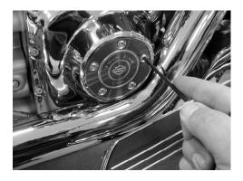
**1.** Remove stock cover using a T20 Torx. Set aside.
