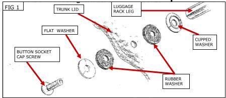
Reinstall the inner surface of the tour box in the same manner as it was removed. Mount the rear half of the rack in the same manner as you did with the front half, except the 10"-24 x 1-1/4" button head cap screws will be used here. Tighten the rear mounting bolts. Do not over tighten the fasteners.
