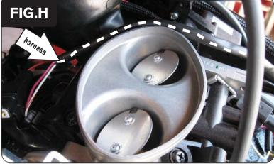
12 Loosen the clamp securing the intake duct to the throttle body. Lift up on the intake duct so the PCFC harness can be routed underneath this duct and in front of the throttle body as shown in Figure H.
