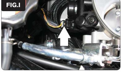
13 Unplug the stock wiring harness from the front injector as shown in Figure I.
