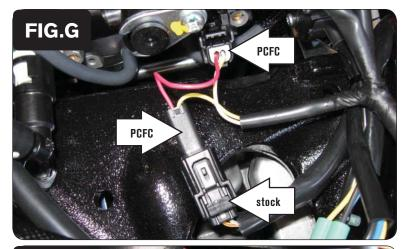
11 Attach the yellow colored wires from the PCFC to the injector and wiring harness as shown in Figure G.
