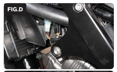
Attach the connectors from the PCFC to the stock wiring harness and throttle body harness as shown in Figure D.
