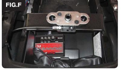
7 Using the supplied velcro, secure the PCFC in the tail section using as shown in Figure F.
