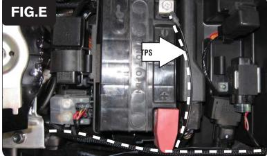
Attach the ground wire from the PCFC to the negative side of the battery as shown in Figure E.
