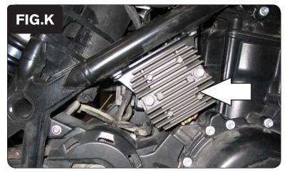
Remove the regulator/rectifier to access the O2 sensor connection as shown in Figure K.
