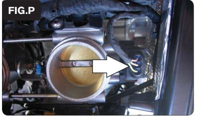
7 Unplug the stock wiring harness from the Throttle Position Sensor (TPS) as shown in Figure P.
