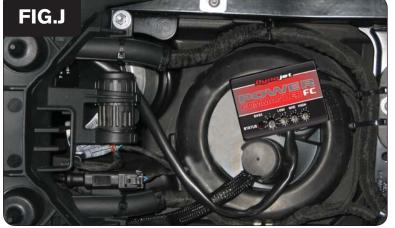
Using the supplied velcro, secure the PCFC as shown in Figure J.
