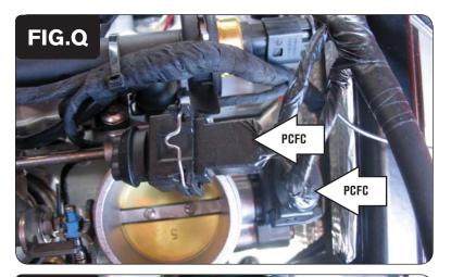
Attach the connectors from the PCFC harness to the stock wiring harness and Throttle Position Sensor as shown in Figure Q.
