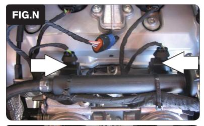
3 Unplug the stock wiring harness from each injector as shown in Figure N.
