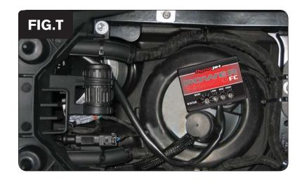
Using the supplied velcro, secure the PCFC under the seat as shown in Figure T.
