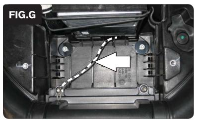
Reinstall the airbox while routing the ground wire from the PCFC through the battery location as shown in Figure G.
