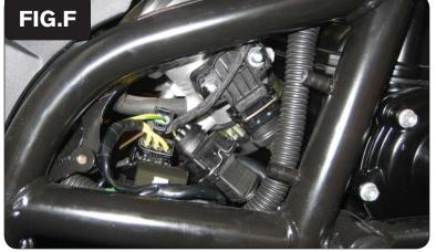
11 Attach the connectors from the PCFC harness to the stock wiring harness and Throttle Position Sensor as shown in Figure F.
