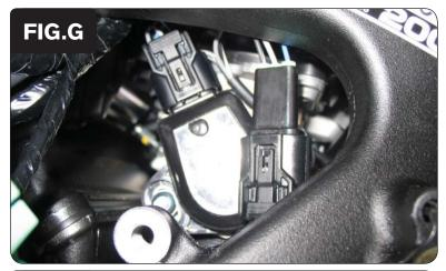
13 Attach the black connectors from the PCFC to the stock TPS and wiring harness as shown in Figure G.
