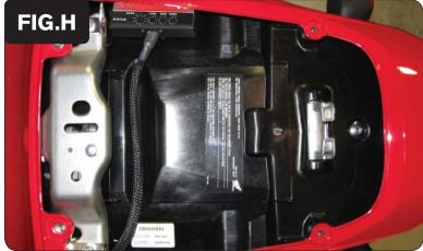
14 Using the supplied velcro, secure the PCFC in the tail section as shown in Figure H.
