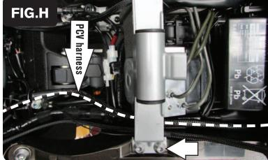
Remove the 4 bolts that hold the fuel tank bracket in place to allow the PCV harness to route underneath it (Fig. H).
