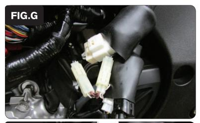
Plug the PCV wiring harness in-line of the CPS and the stock wiring harness (Fig. G).
