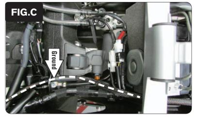
Attach the ground wire of the PCV to the common ground location towards the rear of the engine (Fig. C).
