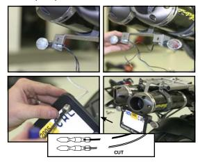
13. Clip wiring to OEM turn signals & plate lights and remove wiring harness from tail section. Remove 2 1/2 in. of outer wiring harness cover to expose wires. Route clipped end of OEM wiring harness through the hole in the new license plate holder and behind license plate frame.
