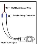
Wrap exposed wiring with electrical tape and secure to plate frame using supplied zip ties.
