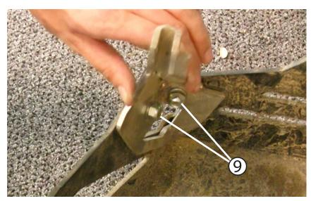
Line up the front left mount bracket as shown, and assemble the hardware in this order: M8 x 25 flat head fastener - finishing washer - washer - locking nut. Do not use thread locker on these fasteners. Do not tighten these down all the way yet.
