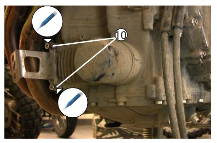
Line up the front right mount bracket and after applying thread locker to the (2) provided M6 x 16 socket head cap screws with washers, use a 5mm allen tool to tighten these all the way down. No need to leave these loose.
