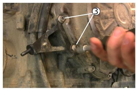
Using a 5mm allen tool, remove these (2) OEM fasteners. Remove the OEM mount bracket. Keep the (2) OEM fasteners handy, you'll be putting them right back.
