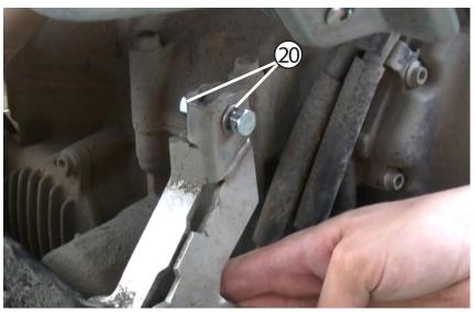
Last, you will tighten this bolt using a 13mm socket and 13mm wrench.
