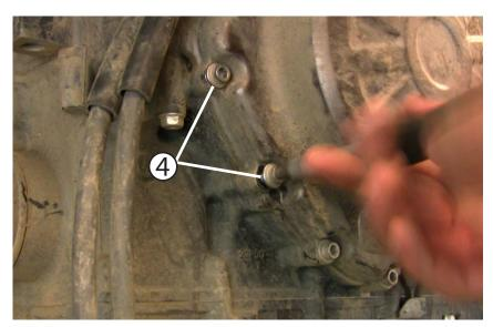
Put the (2) OEM fasteners back and tighten them down.
