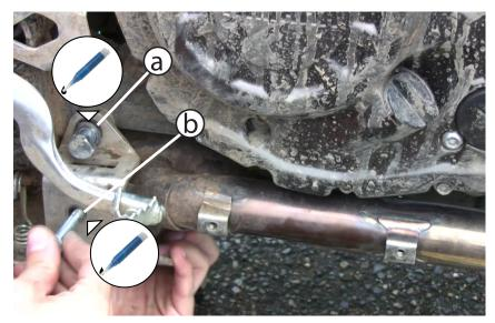
Hold rear mount bracket as shown and: (a) After applying thread locker to both fasteners, use a 17mm socket to start the M10 x 105 fastener and washer. (b) Use a 13mm socket to start the M8 x 45 fastener and washer. Do not tighten these all the way down yet.
