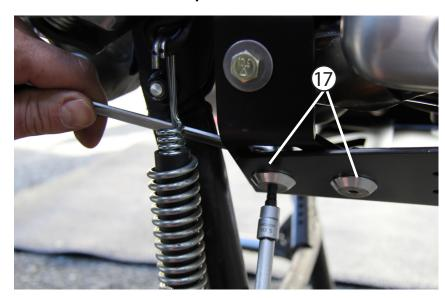
On the right side rear, using a 5mm allen tool and a 13mm wrench, tighten these two fasteners down. Repeat on the left side.
