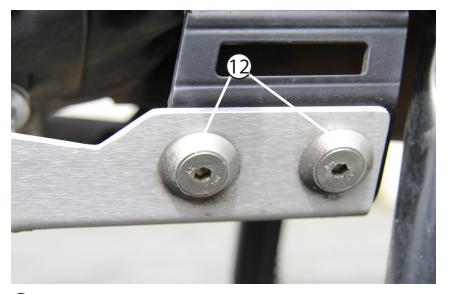
Insert the (2) provided M8 x 25 flat head fasteners, then finishing washers, (on the outside of the plate) then washer, then locking nut and turn them a few turns. Do not tighten these down all the way just yet.
