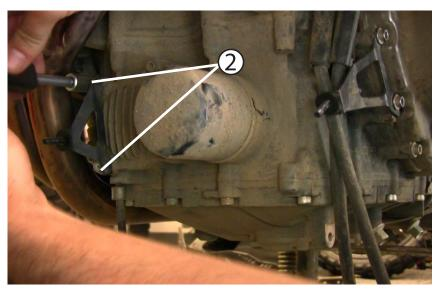
Using a 10mm socket remove these (2) OEM fasteners and remove the mount bracket.
