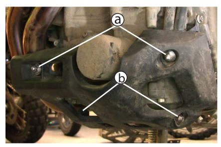
(a) Using a 10mm socket, remove the (2) OEM nuts. (b) Using a 5mm allen tool, remove these (2) OEM fasteners. You will not be reusing any of these.
