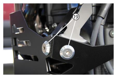
Using a 5mm allen tool and a 13mm wrench, tighten these two fasteners down.
