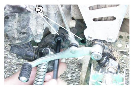
Using an 8mm allen tool, remove these (2) OEM fasteners. Keep them around, you will not be reusing them. When you remove the side stand, a spacer will drop out, you will not be reusing this.
