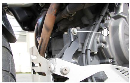
Holding the skidplate up, line up the front left mount bracket with the mount tab shown. Insert the provided M8 x 35 hex cap fastener with washers on each end and get the locking nut started. Do not tighten this down yet. You just want it to hold the plate in place.
