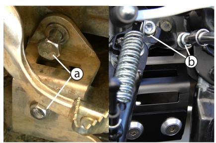
(a) Using a 17mm socket and 13mm socket, finish tightening these bolts down. (b) Using an 8mm allen tool, finish tightening these bolts down.
