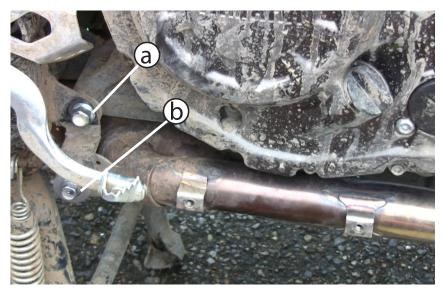
(a) Using a 14mm socket remove this fastener. (b) Using a 12mm socket remove this OEM fastener. You won't be reusing either of these fasteners.
