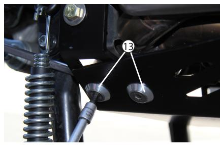
On the right side, insert the (2) provided M8 x 25 flat head fasteners, then finishing washer, (on the outside of the plate) then washer, then locking nut and turn them a few turns. Do not tighten these down all the way just yet.
