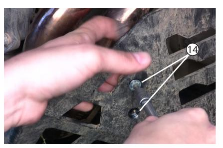
Insert the (2) provided M6 x 18 flat heads, washers and locking nut and using a 10mm wrench and 4mm allen tool, start tightening these. Do not tighten them all the way down yet. We'll keep this a bit loose for now.
