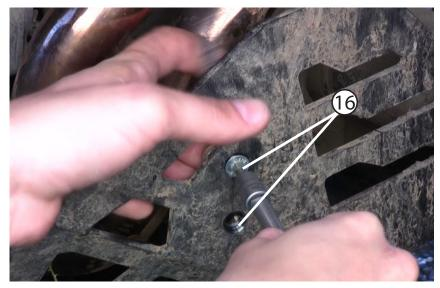
Now come back to the front left bracket and using a 10mm wrench and 4mm allen tool, tighten these down.
