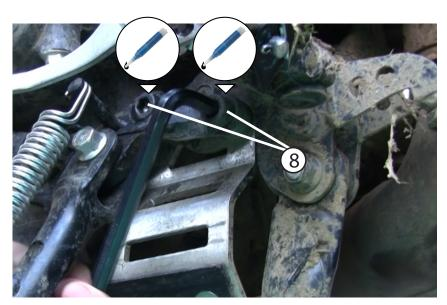
Put the sidestand back up to its mount holes. You no longer need the spacer that came out when you removed the OEM bolts. Apply thread locker, then using an 8mm allen tool, insert and tighten these (2) provided M10 x 40 bolts with the (2) remaining M10 washers a few turns. Do not tighten all the way down yet.
