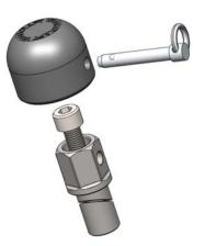
A note for racers: If your tech inspector wants you to safety wire these (most will not) then you simply need to orient the pins so that the pull on the pin is both clockwise and down (so that it acts to tighten the bolt and pull the pin into the puck)
