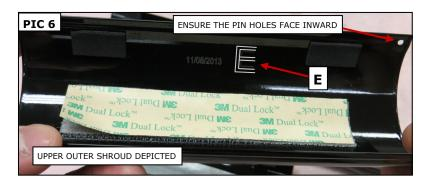
STEP 10 Refer to PIC 8 and 9. Test fit the Upper Outer (**E**) and Upper Inner (**F**) Shrouds on the brake-side (right) fork.
