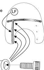
Line up the Right rear strap with the right set of vertical holes on the rear of the windshield. The step on the right rear strap sits over the 5 hole rear strap.
