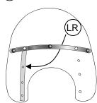
5. Line up the Left front strap with the left set of vertical holes on the front of the windshield. Push a large socket spacer through the left front strap, and into the holes in the windshield, at the locations shown. Push a cap screw through each spacer and through the Left rear strap. Slide a plastic spacer washer over the protruding threads and secure loosely with an acorn nut.
