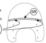
3. Line up the 5 hole front strap with the horizontal holes on the front of the windshield. Push a large socket spacer through the front strap, and into the holes in the windshield, at the locations shown. Push a cap screw through each spacer and through the 5 hole rear strap. Slide a plastic spacer washer over the protruding threads and secure loosely with an acorn nut.
