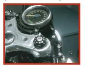
3. Drop in the RSD riser plugs into the holes on the upper triple clamp.
