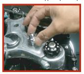
4. Install the supplied 3/8" button head screw, flat washer, and lock washer from the underside of the triple clamp and torque to 15 ft-lbs.
